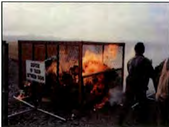
Figure 15. Open burning method - Burn cage
